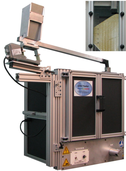
Figure 7. Segregation tester used to measure the segregation pattern of the material
