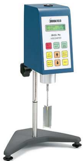
Figure 2. Vane viscometer used in experimental tests
