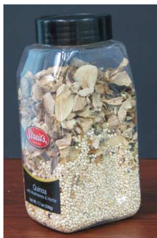
Example of segregation by PSD difference with quinoa and dehydrated mushroom mix
