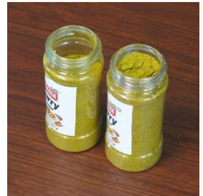
Example of density variation due to cohesiveness and/or strength of bulk powder with curry seasoning
