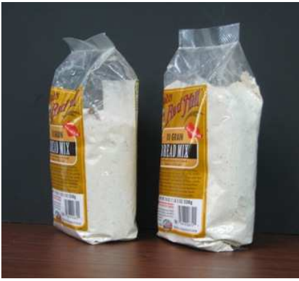
Example of density variation due to air entrained in product during packaging which allows post-fill settling of bread mix
