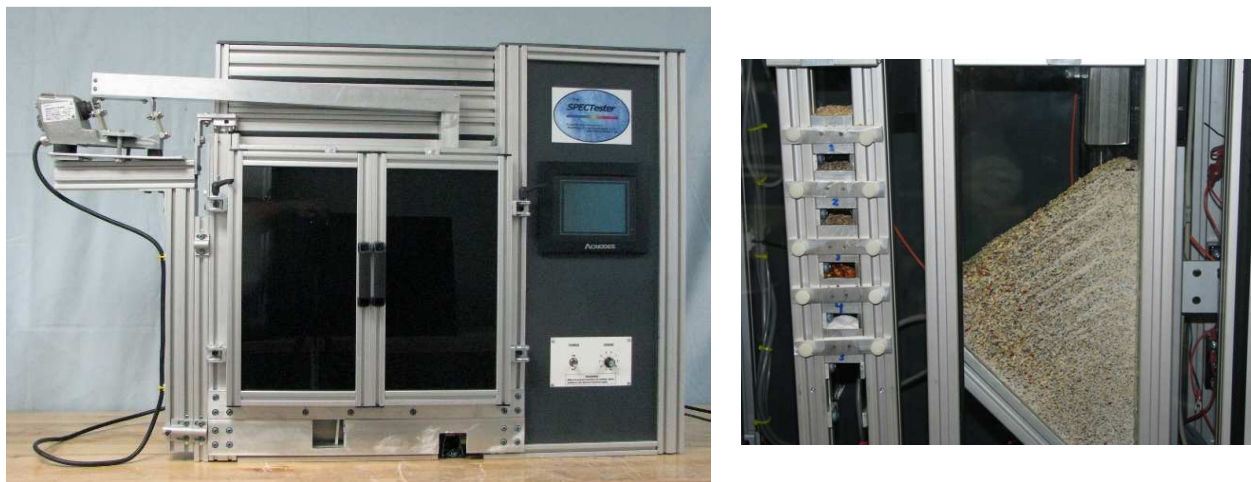
Figure 3. Segregation tester used in experiment showing the variable speed vibratory feed system and the pile formed in the tester for analysis (note right door is open to expose the segregation hopper)
