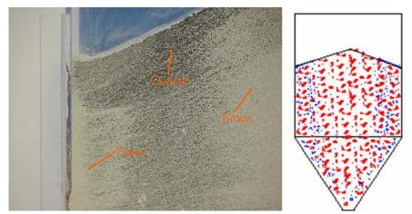
Fig 3. Typical air entrainment segregation
