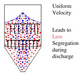
Fig 6. Mass flow profile with radial segregation pattern.
