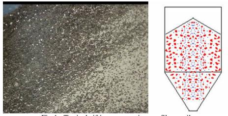
Fig 1. Typical sifting segregation profile on pile
