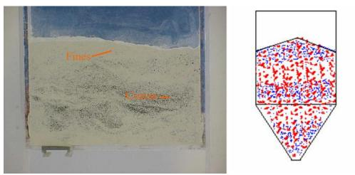
Fig 4. Typical impact fluidization segregation
