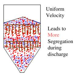
Fig 5. Mass flow velocity profile with impact fluidization segregation profile.
