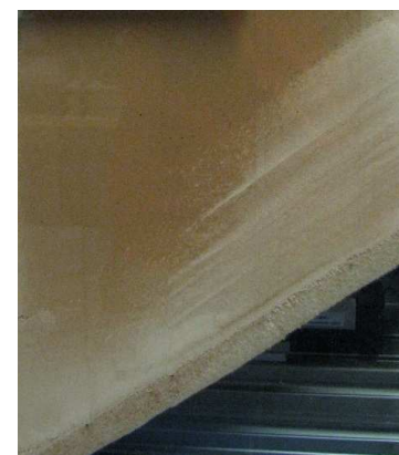
3-component blend (dry milk, sugar, cocoa powder) showing air entrainment segregation issues
