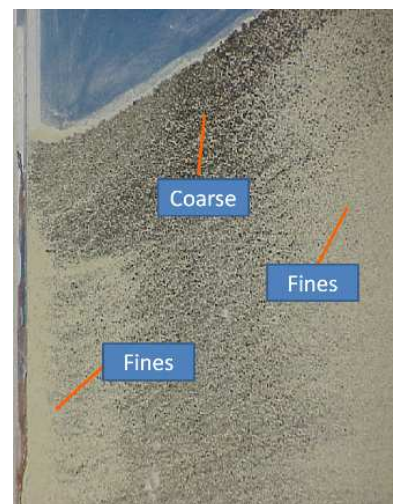
Figure 3. As gas currents diminish, fine particles are deposited, resulting in air entrainment
