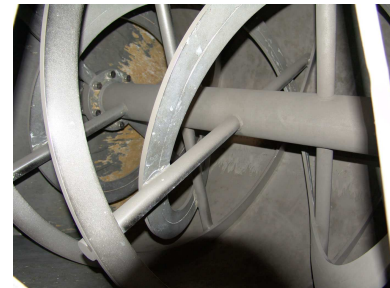
Figure 4. A rotary blender – best considered to reduce segregation resulting from air entrainment.
