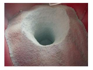
Material hang-up (arching and/or ratholing) problems are generally caused by one of four things: cohesive forces between powder particles or granules, external forces, inter-particle locking, or elastic constraint issues. It is critical to understand the type of hang-up that you may be experiencing.
