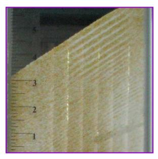
Segregation occurs through several mechanisms. Identification of the primary segregation cause and the segregation pattern produced through handling is critical to *prevent segregation* (or demixing) of the final mixture during handling and packaging. Any property difference between materials can cause separation of critical material components. However, there are five common causes of segregation problems in typical handling systems:
