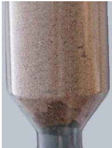
Arch across hopper opening
