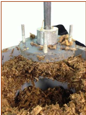
Wet biomass as it shears under applied stress load in a large (12") uniaxial test cell
