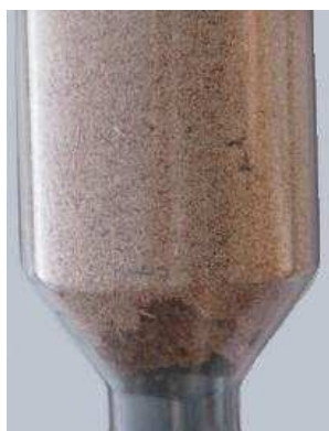
Figure 2: Arch of biomass in typical (improper design) storage hopper
