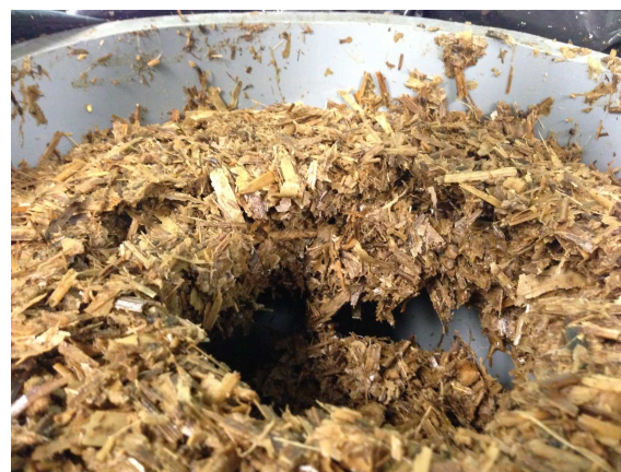
Figure 3. Strength of wet biomass is characterized in a large-cell uniaxial test cell
