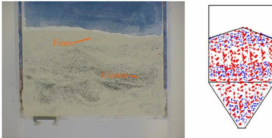
Fig 4. Typical impact fluidization segregation
