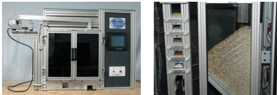
Figure 1. SPECTester used in experiment showing the variable speed vibratory feed system and the pile formed in the tester for analysis (note right door is open to expose the segregation hopper)
