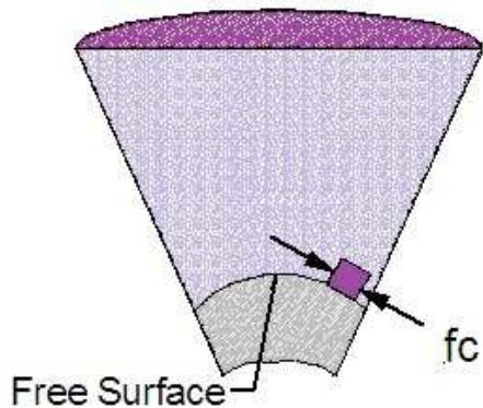
**Cohesive flow problems** are one of the main reasons a plant handling a bulk material fails to operate. When it is not possible to design a material free of integral cohesive flow properties, the system must be designed to handle the problem. Cohesion is a function of the unconfined yield strength of bulk material (fc).
