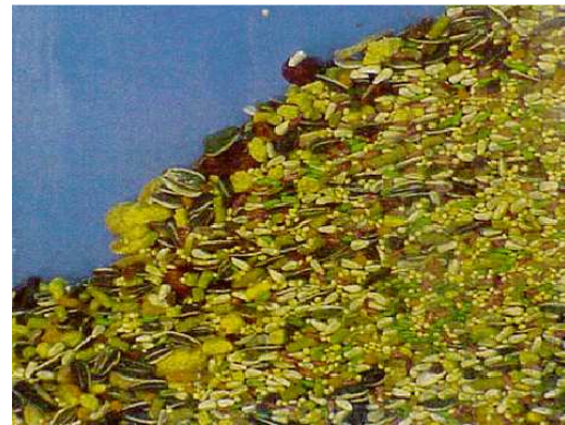
Figure 3. Segregation patterns formed during pile formation in a process
