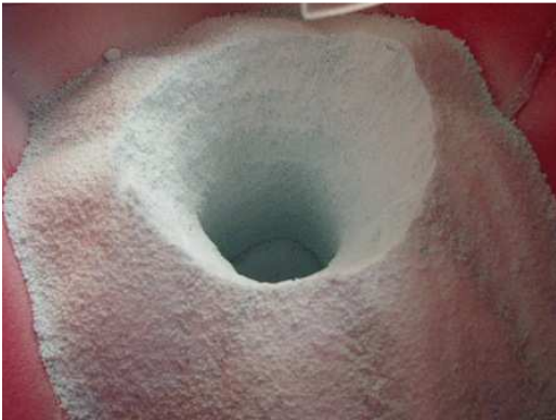
Figure 2. Material hang-up (rathole and arching) of material in a system causes process down-time
