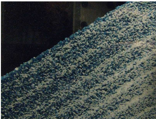
Figure 3. Segregation patterns formed during pile formation in a process
