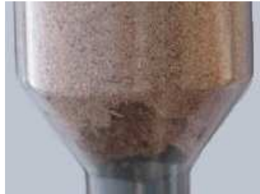
Figure 2. Material hang-up (rathole and arching) of material in a system causes process down-time
